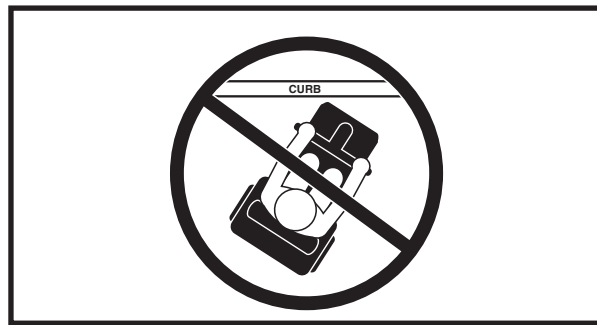
Figure 7. Incorrect Curb Approach
